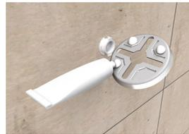
3. Apply flexi-fix adhesive to the wall plate.
